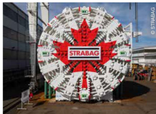
Tunnelbohrmaschine Diggy Scardust
