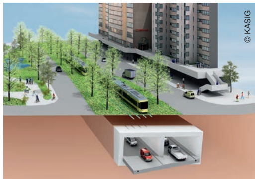
Two-lane car tunnel
