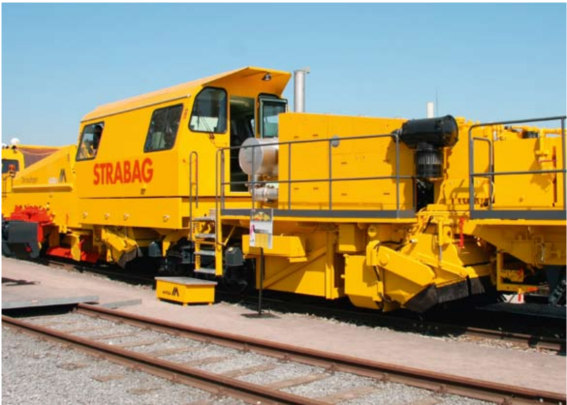
THE R24 BALLAST REGULATOR SHAPES AND DISTRIBUTES TRACK BALLAST AT 2 KM/H
