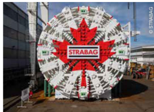
Tunnel boring machine Diggy Scardust.
