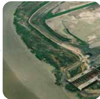
Center: Construction of tunnel element Right: Preparations for the floating of tunnel element Below: Drydock for tunnel element construction and settling tank for the excavated material
