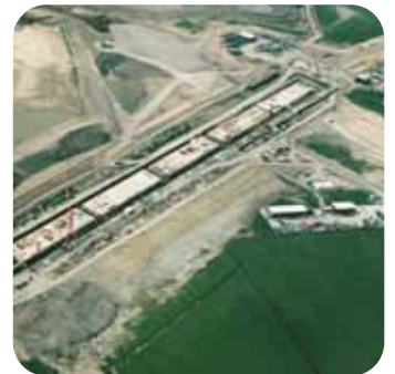
Center: Construction of tunnel element Right: Preparations for the floating of tunnel element Below: Drydock for tunnel element construction and settling tank for the excavated material
